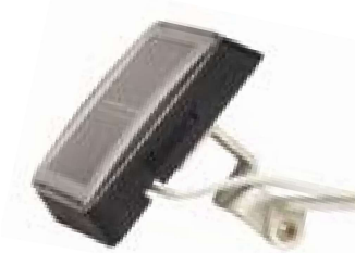
SPNODE Solar Panel Kit (optional) Height: ¾" Length: 3" Width: ⅝" Controller to solar panel: 100' maximum 18 AWG direct-burial wire
