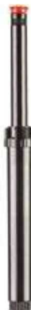
PSU-06 Retracted height: 9½" Pop-up height: 6" Exposed diameter: 1¼" Inlet size: ½"
